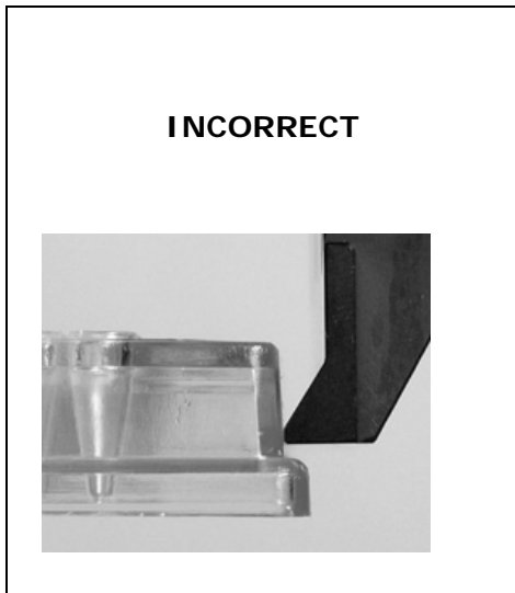
Figure 94: Incorrect Positioning of the Dogs
