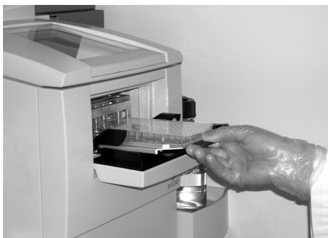
Figure 3-9. Loading the rack tray into the sample compartment.
