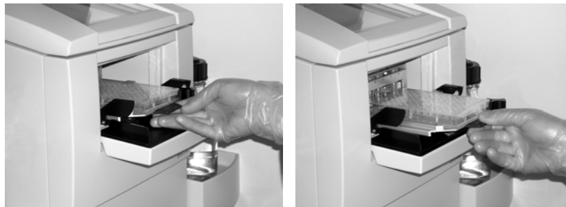
Figure 3-5. Removing the rack tray from the instrument.
