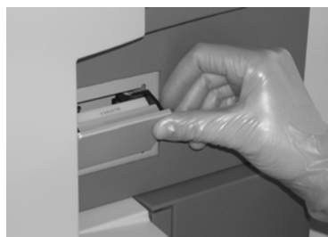
Figure 2-5. Inserting a sensor chip.
