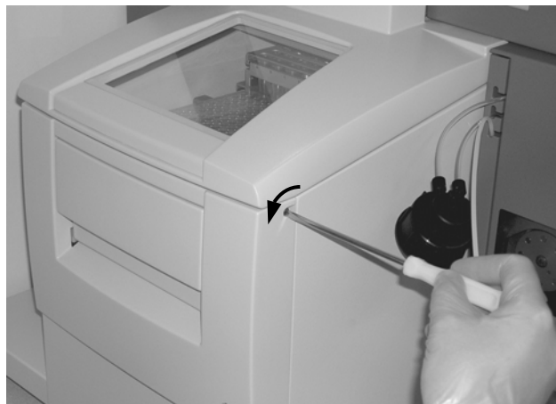
Figure B-8. Opening the sample compartment door.
